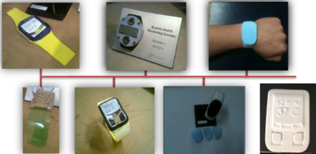
Figure 4. Typical physical prototype evolution from the medical device project
