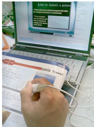
Figure 2-1 : User point the G-Scanner on any printed text or picture in the textbook to activate e learning on the Computer.
