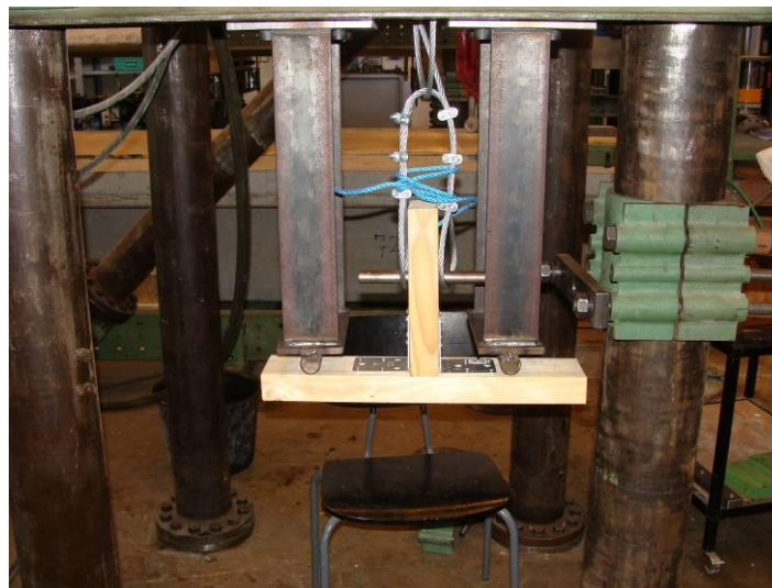
Figure 3. Testing 1:1 timber joint
